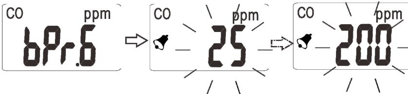
The alarm beeper prompts personnel to evacuate an area because of the detection of unsafe concentrations of CO. The meter alarms when the CO concentration exceeds the default or user-programmed threshold.
